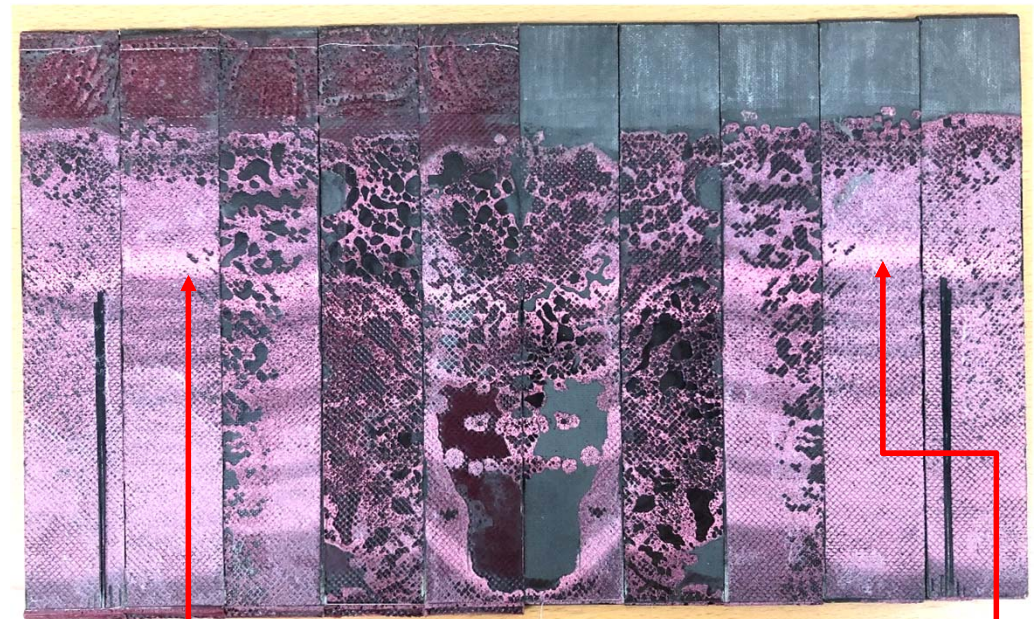
Crack growth region during wedge testing
